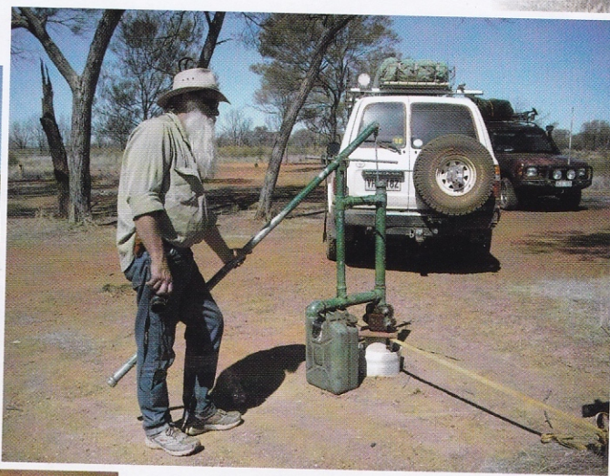
Above: Rob with the repaired pump on Lynette's Bore at Camp Beadell.
